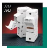
US3J & US6J **Modular Holders** 600V AC 30 & 60A Class J **UL Listed** Meet the requierement of UL512 Finger Safe **Optional Indicating Lights** DIN Rail Mount Compact footprint Quick, easy fuse change.
